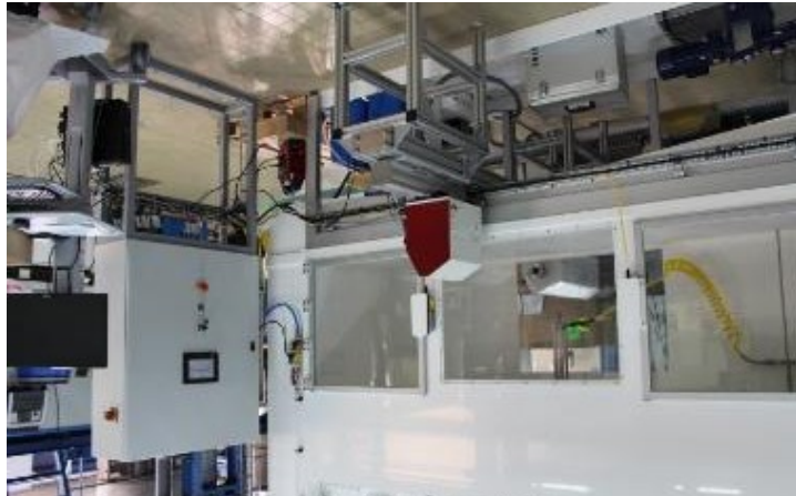
Spray chamber with Sympatec laser for droplet size distribution assessment
